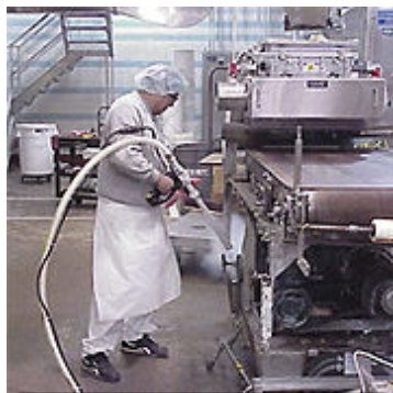
Dry ice blasting used to clean bakery equipment
