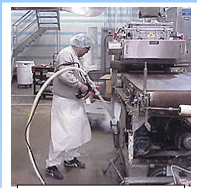
Dry ice blasting used to clean bakery equipment
