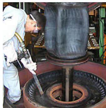
Dry ice blasting used to clean a rubber mold
